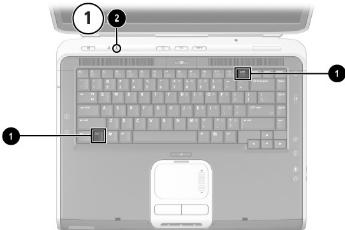
Identifying the Fn and num lock keys and the num lock light
