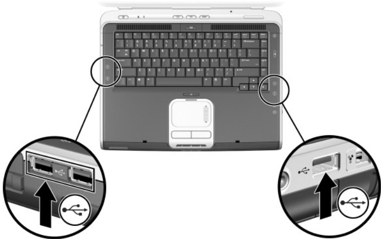
Identifying the two USB connectors on the left side and the one USB connector on the right side
